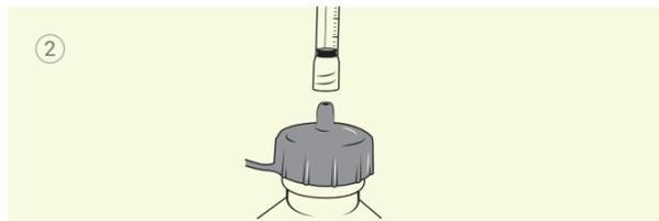
**Step 2.** Attach syringe to the bottle adapter.
