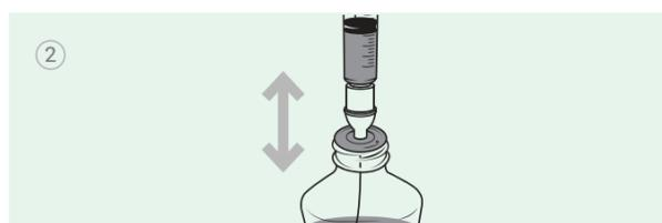
**Step 2.** Insert straw, cycle syringe to eliminate air bubbles. Draw up desired dose.
